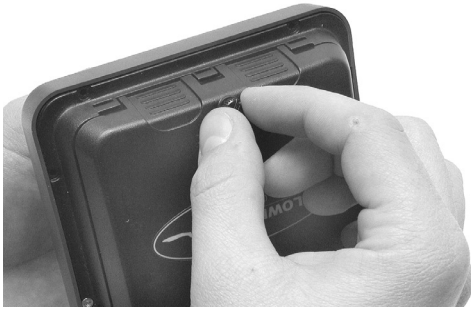
Loosen thumbscrew and remove AirMap battery cover.
